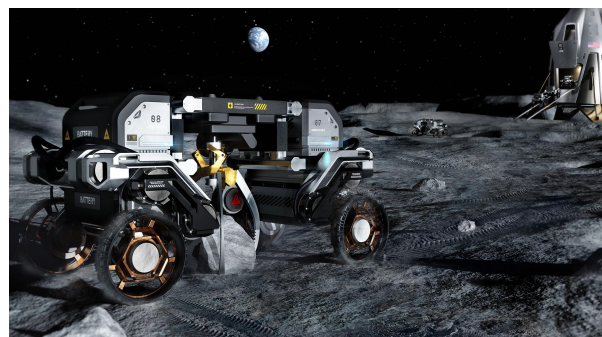
Figure 4. The Armstrong UMV concept with chassis in “arch” configuration and with a gripper tool to clear rocks from the surface.
